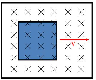
*Nope*, the magnetic flux is NOT CHANGING through the face of the coil, so there is no induced EMF set up in the coil.
