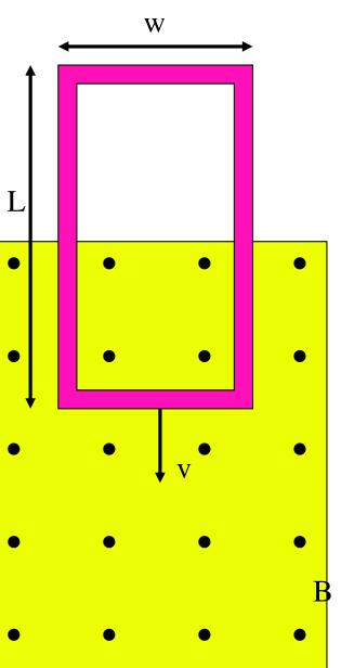
A loop of mass m, resistance R and dimension w and L falls from rest into a B-field. During the time interval before the top edge of the loop reaches the field, the loop reaches terminal velocity.
