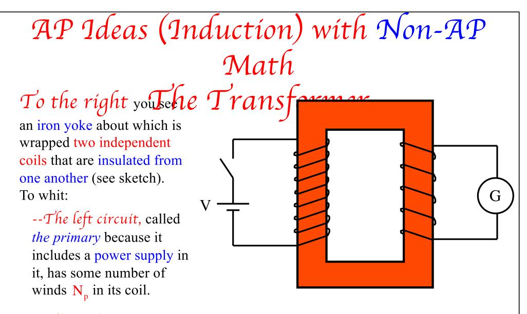
*--The right circuit*, called *the secondary* because it includes a device you are transferring power to, has some number of winds  $N_s$  in its coil.
